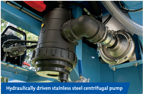
Hydraulically driven stainless steel centrifugal pump
